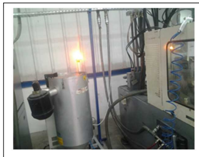
Figure 8. Inappropriate storage of the thermoplastic resin.
