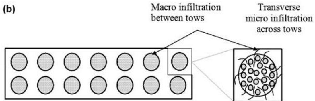
FIG. 6. (a) Interbundle versus intrabundle infiltration and (b) principles of macro- and microinfiltrations.
