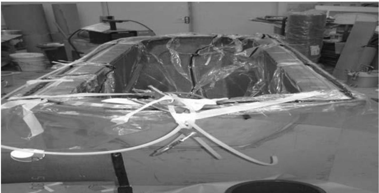
FIG. 5. The resin and vacuum lines set up.
