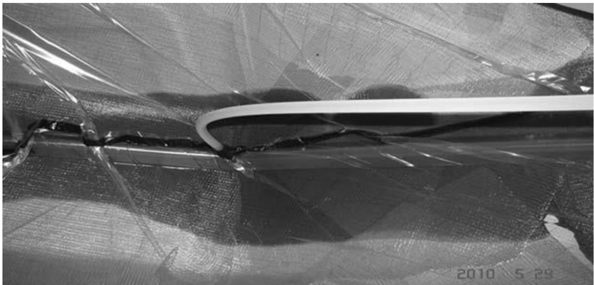
FIG. 7. The initial phase of resin infusion shown by dark green color.
