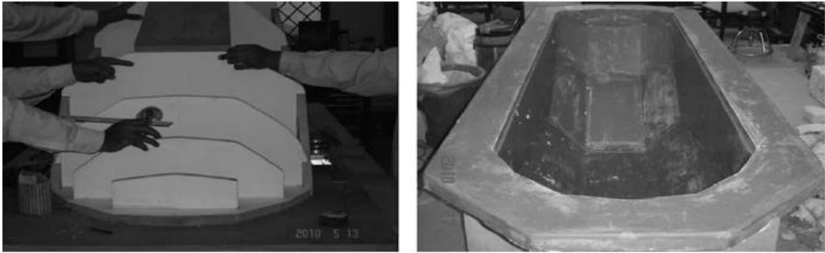
FIG. 3. The pattern (LHS) and mold (RHS) ready for resin infusion manufacturing process.
