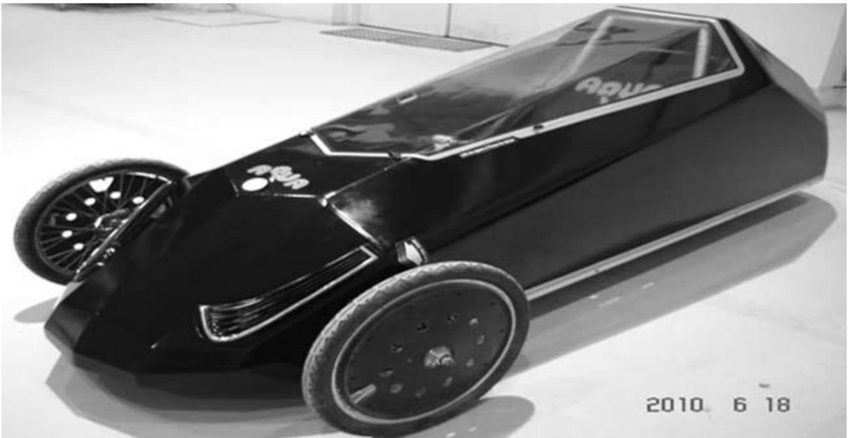
FIG. 11. The all composite car body ready to take part in Shell Eco Marathon.
