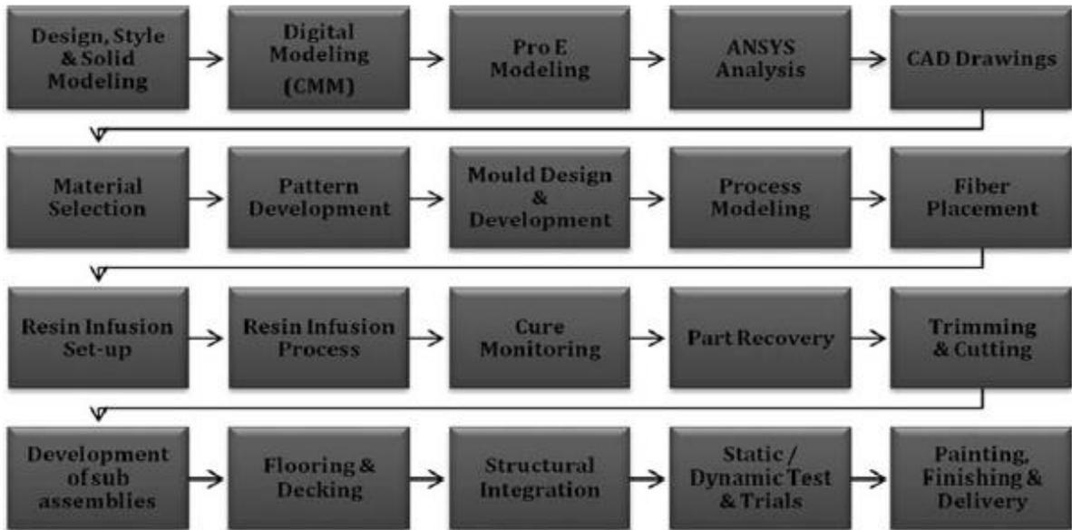
FIG. 4. The sequence of development of car body through single-step resin infusion.
