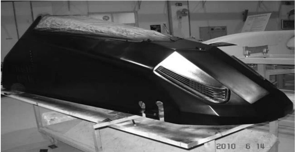
FIG. 10. The All composite integrated car body showing cockpit, air inlet, and engine access door.
