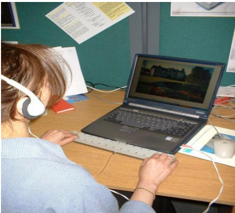
Figure 7 The developed 128x4 interactive interface graphical tactile display prototype using ABS and ER fluid technology
