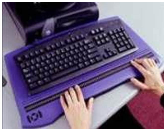
Figure 1 One row form electronic refreshable graphical tactile display for the visually impaired and blind access to information technology resources [1-5]
