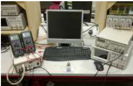
Figure 10: Practical test rig arrangement used to measure the characteristics of the fabricated 3D USM actuator prototype using single flexural vibration transducer
