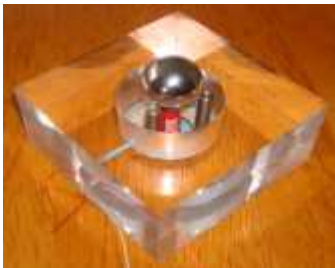
Figure 8: Fabricated Prototype of the proposed 3D USM using a single piezoceramic flexural vibrating ring transducer
