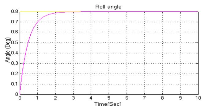
Figure 10: Roll Fuzzy-PID design response
