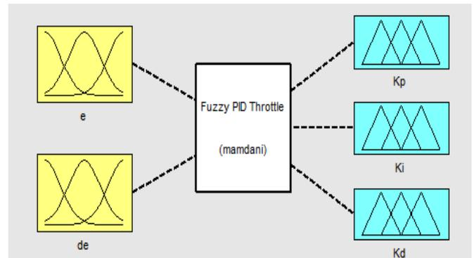
Figure 4: Basic structure of a fuzzy-PID controller for throttle
