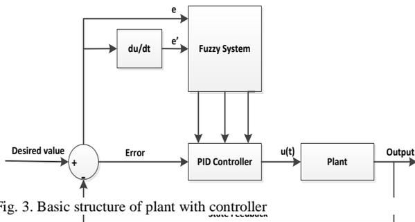
Fig. 3. Basic structure of plant with controller
