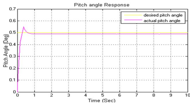
Figure 11: Pitch angle PID design response
