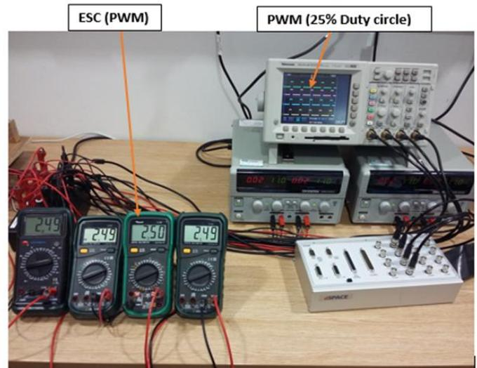
Figure 13: Real-time interface wave generation for quadrotor
