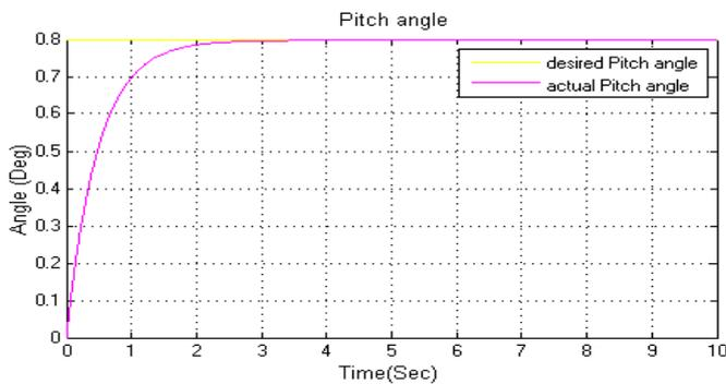
Figure 12: Pitch Fuzzy-PID design Response
