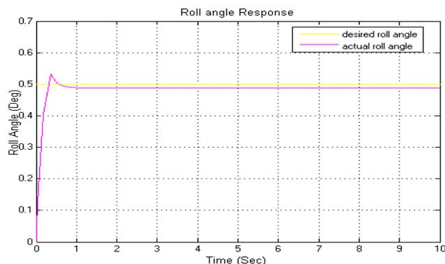
Figure 9: Roll angle PID design response
