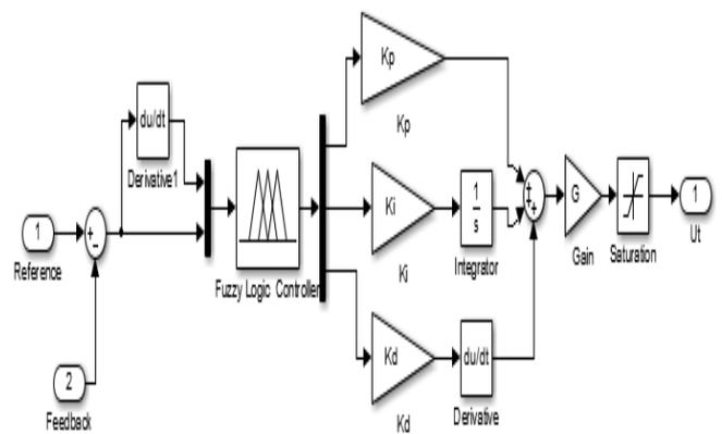
Figure 6: General controller for Throttle, Roll and Pitch
