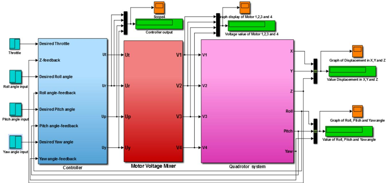
Figure 7: The complete non-linearized dynamic quadrotor Simulink model
