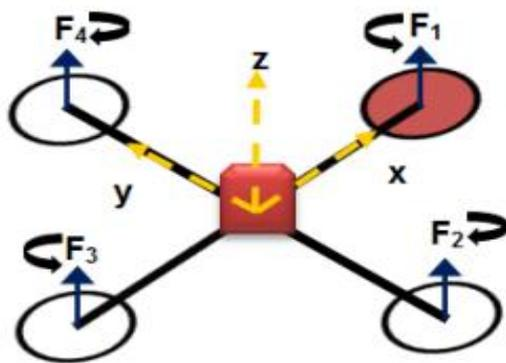
Figure 1: Inertial and Body Fixed Frame
