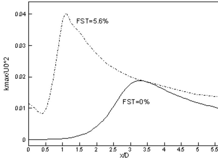
**FIG. 10.** Development of the maximum turbulent kinetic energy; LTL-case (solid line), ETL-case (dashed line)
