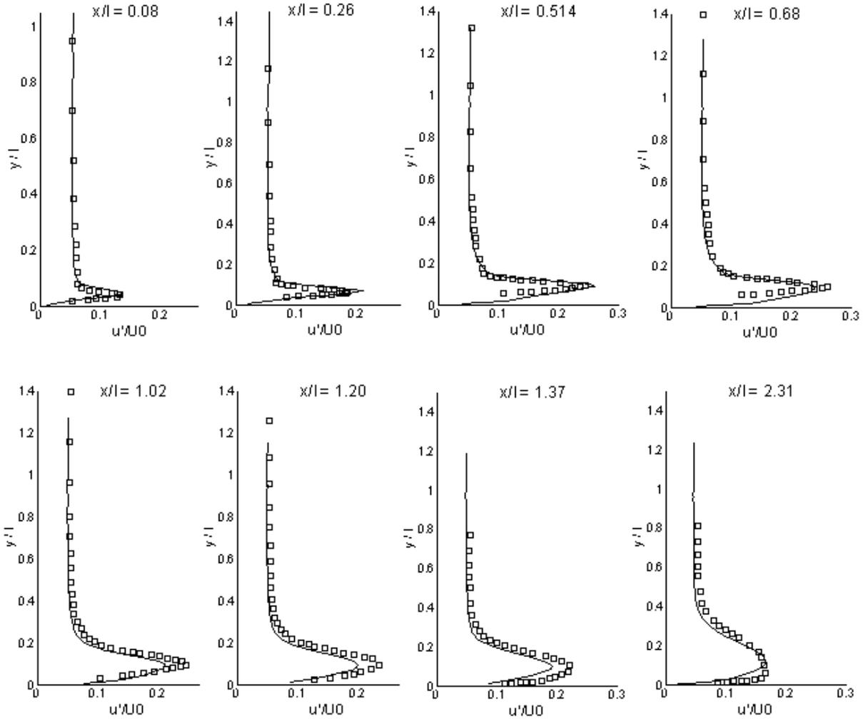
**FIG. 7.** rms streamwise velocity fluctuation  $u'$  at different streamwise stations (ETL-case), Present LES (solid lines), Exp. Data (symbols)
