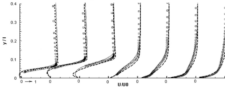
**FIG. 4.** Mean streamwise velocity at seven streamwise stations (LTL-case), Left to right:  $x/l = 0.22, 0.44, 0.66, 1.09, 1.27, 1.64, 2.55$ . Present LES (dashed), LES of Yang & Voke [2] (solid line), Exp. Data (symbols)
