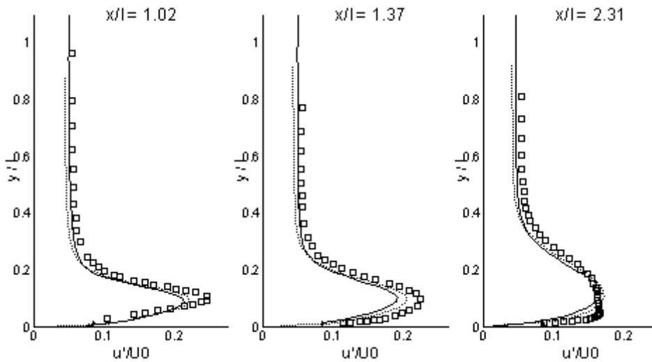
**FIG. 8.** rms streamwise velocity fluctuation  $u'$  at different streamwise stations (ETL-case), coarser grid (solid lines), refined grid (dotted lines), Exp. Data (symbols)
