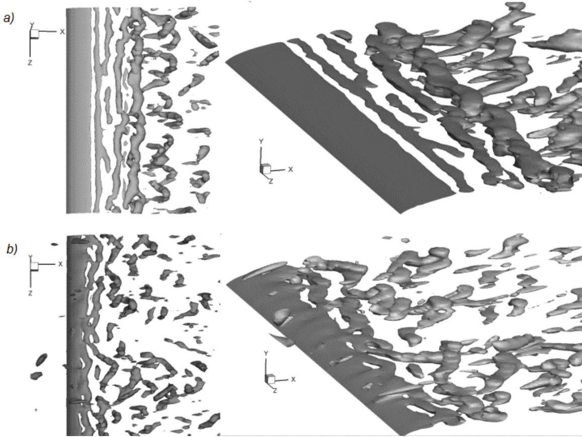
**FIG. 13.** Top and perspective views of the Q-criterion isosurfaces; (a) LTL-case, (b) ETL-case
