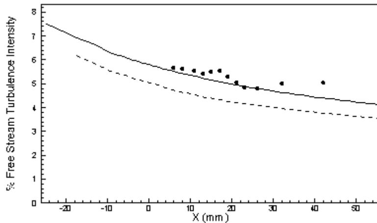
**FIG. 3.** Decay of free-stream turbulence intensity for ETL-case (5.6% at leading edge), Soling line:  $y/D = 4.0$ ; Dashed line:  $y/D = 1.5$
