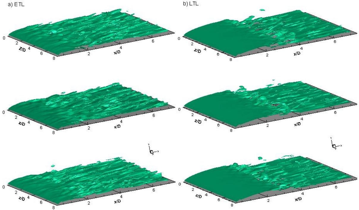
**FIG. 9.** Isosurfaces of instantaneous spanwise vorticity at three different time;
