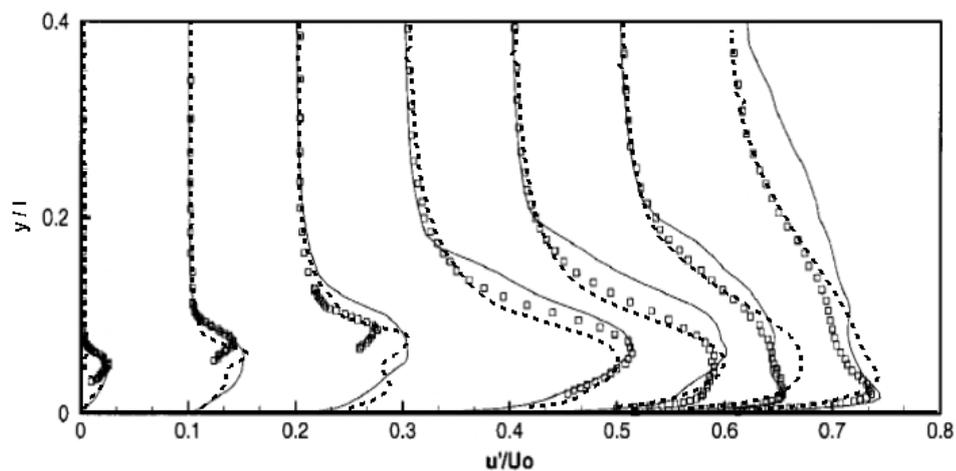
**FIG. 5.** rms streamwise velocity fluctuation  $u'$  at seven streamwise stations (LTL-case), Left to right:  $x/l = 0.22, 0.44, 0.66, 1.09, 1.27, 1.64, 2.55$ . Present LES (dashed), LES of Yang & Voke [2] (solid line), Exp. Data (symbols)
