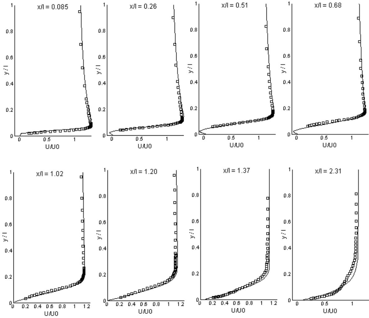
**FIG. 6.** Mean streamwise velocity at different streamwise stations (ETL-case), Present LES (solid lines), Exp. Data (symbols)
