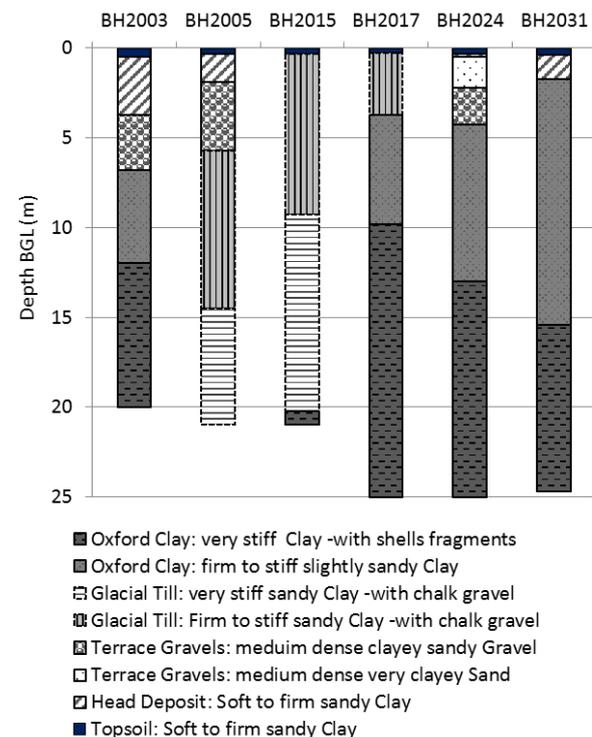
Figure 3 Borehole logs showing the geology of the site where the CPT trial has taken place.
