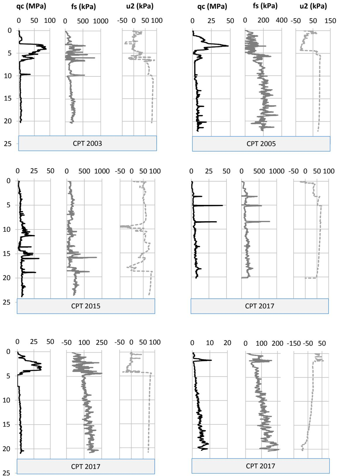
Figure 4 The measurements of CPTUs: Tip Resistance  $q_c$ , Sleeve Resistance  $f_s$ , and Pore Pressure  $u_2$ .
