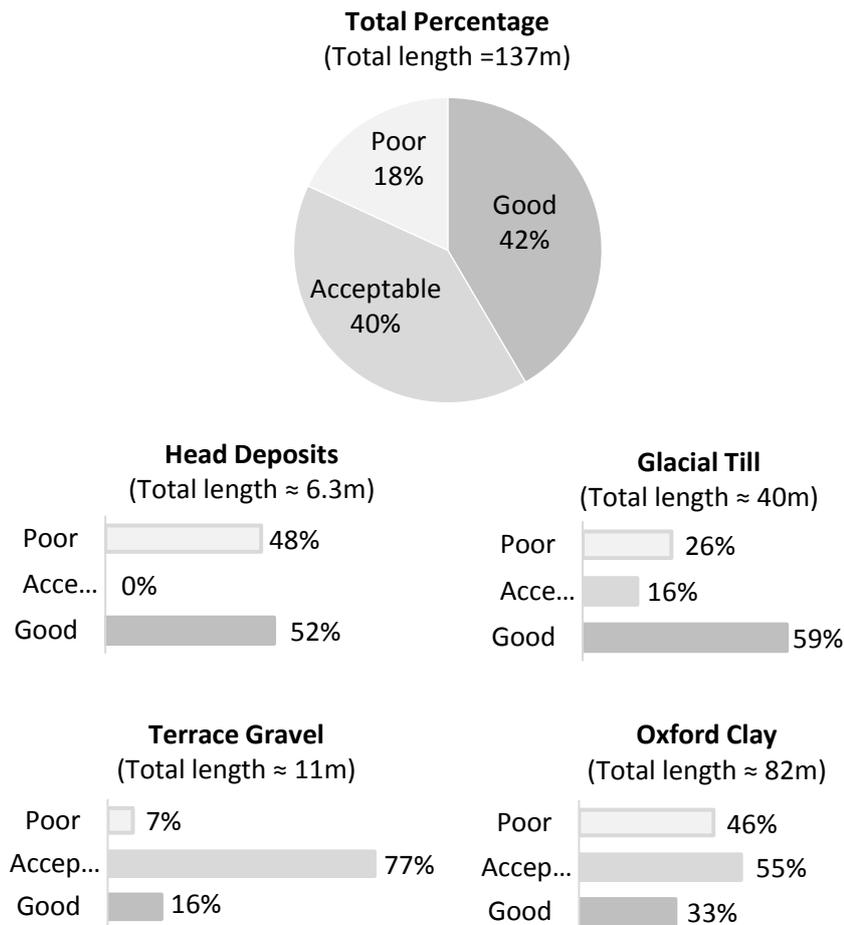
Figure 5 Percentage of the level of agreement between BH-based and CPT-based soil types.
