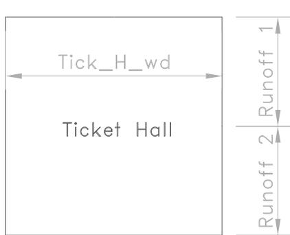
The ticket hall in figure 4 highlights the two factors that determine its length and width in the SGEvac software. The Tick\_H\_wd (ticket hall width) is the parameter taken directly from site specific flow figures, and both run-offs are given as a set 6 metres to generate an initial shape. A 6m distance is used since the Standard for the UTS gateline (taken as the centre of the ticket hall) to street level is a 6m distance, and so is the UTS gateline to a staircase.
