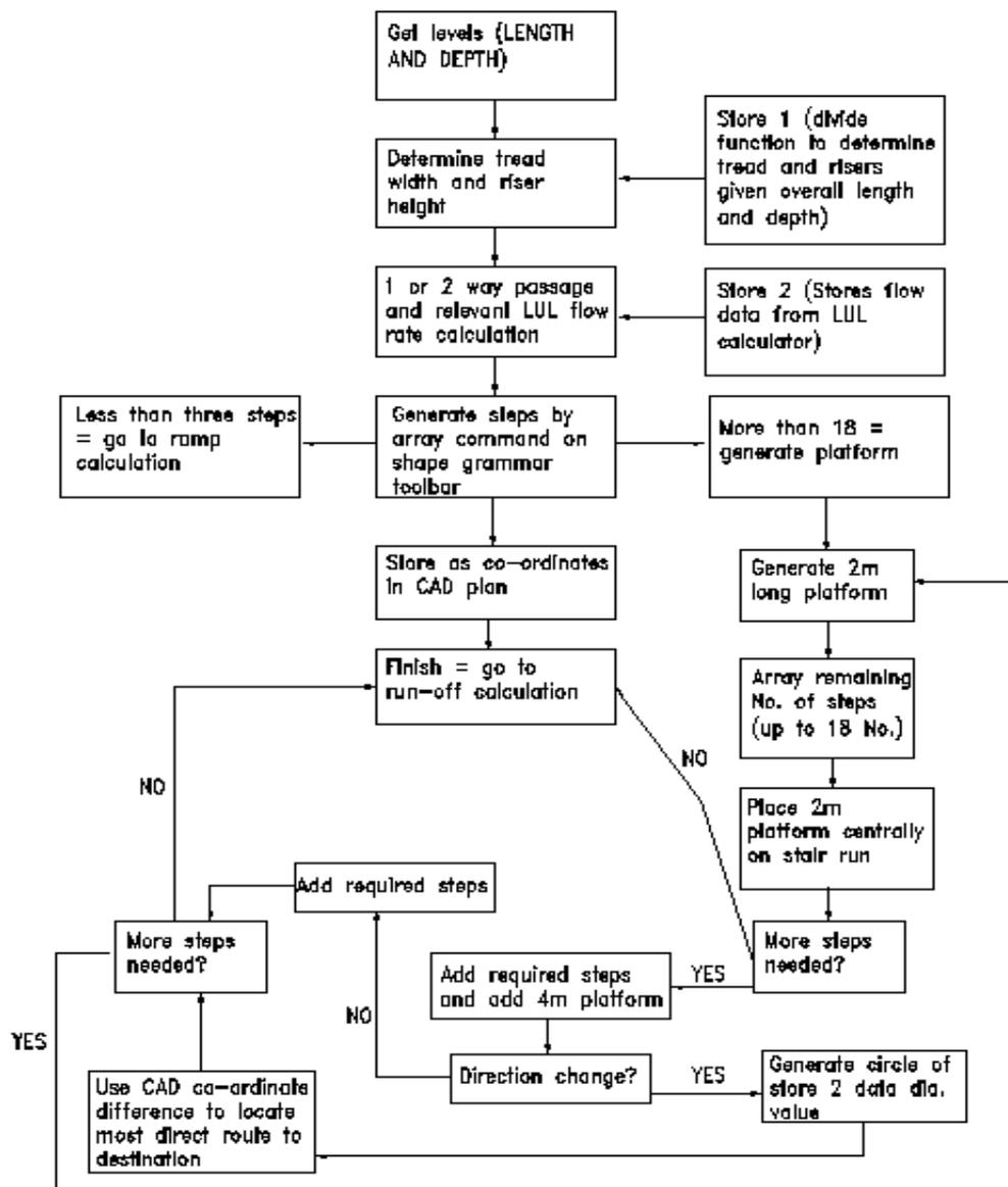
Figure 8 – Stair SGEvac generation method
