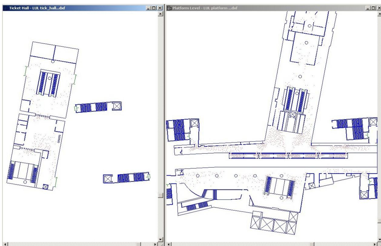
**Figure 11 - Station Evacuation after 25 seconds in SIMULEX software**
