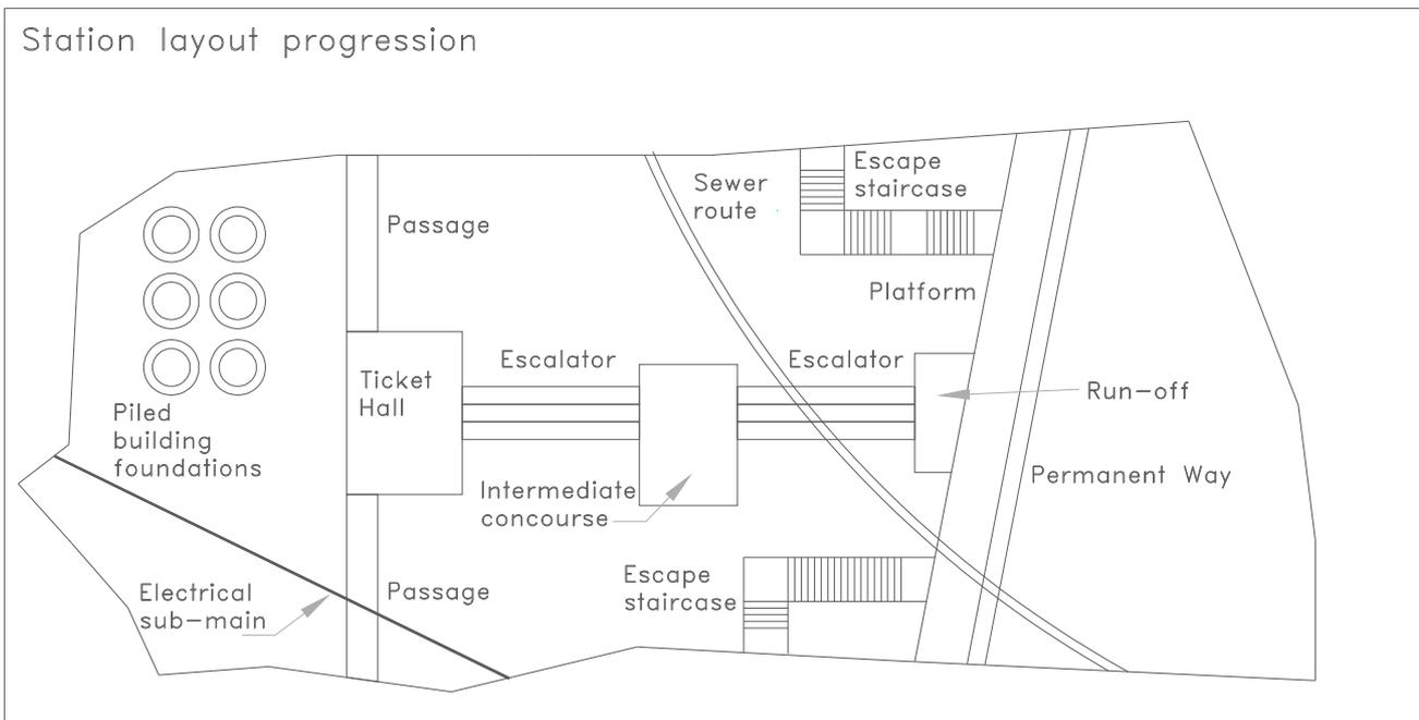
**Figure 10 – SGEvac Station Layout Progression showing site constraints**
