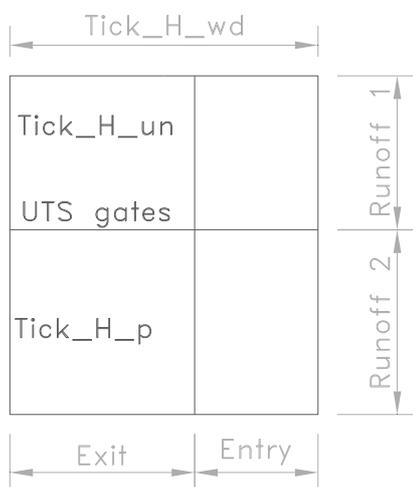
Figure 5 is an advancement from figure 4 where run-off No. 2 has been lengthened to accommodate an escalator run-off (say 10m in this example for a medium flow station), the UTS gateline (centre line) has been inserted and Tick\_H\_un (unpaid side of the hall), and Tick\_H\_p (paid side) have also been defined (and the ticket hall thus orientated on the site overall by the paid side of the ticket hall also being trackside to ensure LUL obtains revenue).
