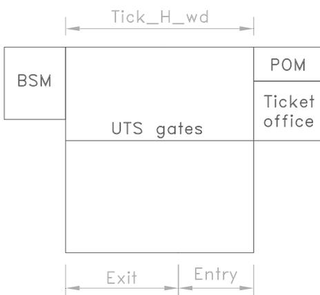
Figure 6 demonstrates addition rules. The logical position for the ticket office (sized by regulations as 11m<sup>2</sup>/per staff member) is to the unpaid side of the ticket hall, as is the POM (passenger operated machine) enclosure. The BSM (Business Station Manager) office can be located on the unpaid or paid side of the ticket hall.
