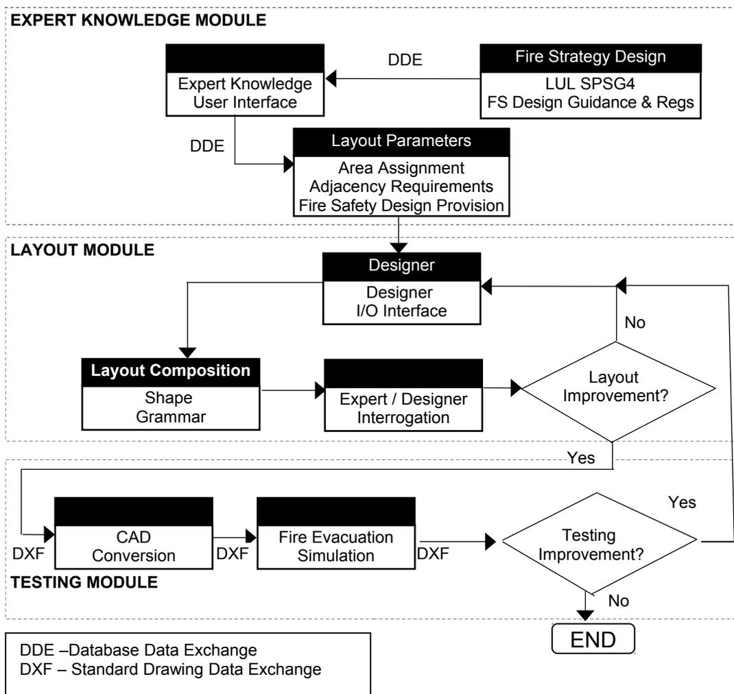
Figure 1 – Proposed SGEvac System Algorithm
